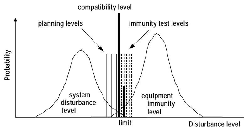
**Figure 1 — Illustration of the concept of compatibility levels**
